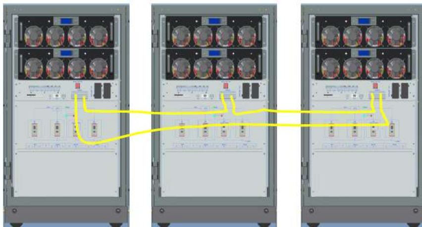
The signal cable connection for 3 UPSs in parallel
