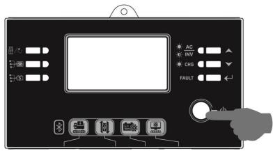
Once the unit has been properly installed and the batteries are connected well, simply press On/Off switch (located on the LCD module) to turn on the unit.
